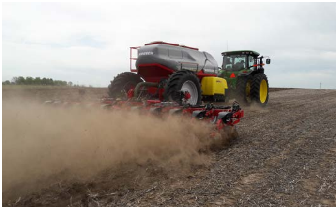
Figure 2. Dust behind a pneumatic planter during planting which may contain residual seed lubricant and seed treatment coatings.
