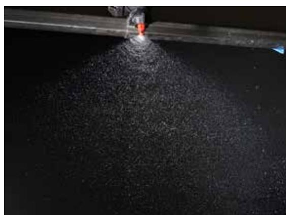
*Figures 1-3. These images show the difference in droplet size based on the type of nozzle selected. Nozzle: AIXR 11004 (air inclusion 110-degree flat fan coarse spray); XR11004 (flat fan medium/fine spray); and TTI04 (Turbo Teejet Extra coarse spray). Photo: Mark Ledebuhr, Application Insights, LLC 2020, [www.bugwood.org](http://www.bugwood.org)*
