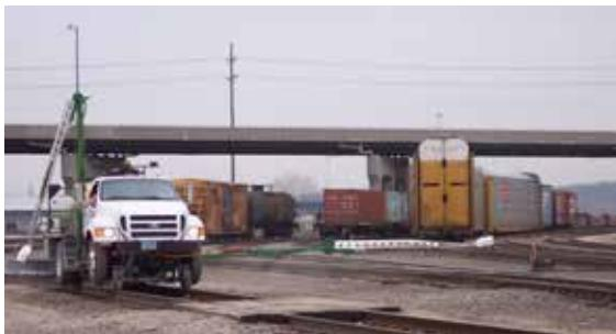
*Figure 8. Trucks with the ability to move on roads or rail are commonly used to treat railroad ballasts.*
