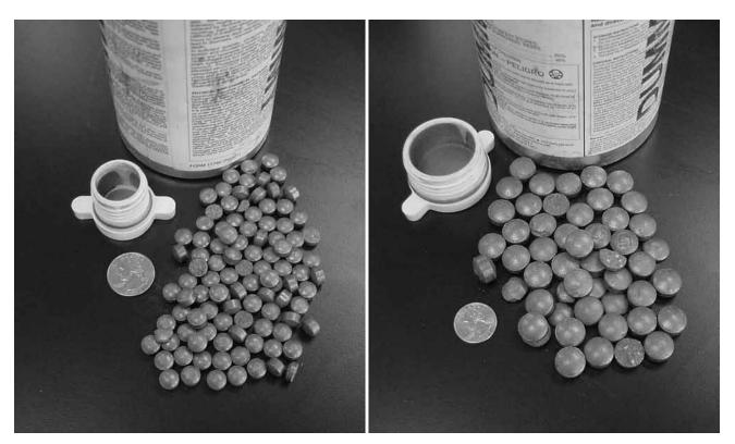
Figure 3. Pellets (left) and tablets (right) of aluminum phosphide that generate 0.2 and 1.0 g, respectively, of phosphine each when fully reacted.
