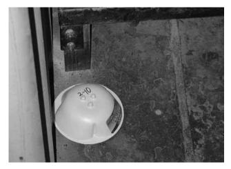
Figure 4. Trap for monitoring insects on mill or warehouse floors.
