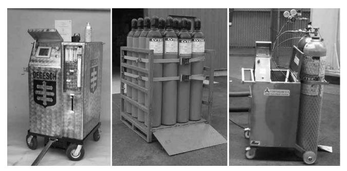
**Figure 4.** A phosphine generator (left). Cylinder-based phosphine at 2% in carbon dioxide (center) and 100% PH<sub>3</sub> being diluted immediately in air (right).
