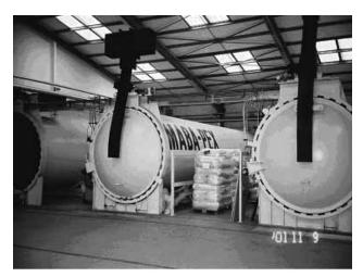
**Figure 2.** Application of high pressure CO<sub>2</sub> for the dry fruit industry in Turkey.
