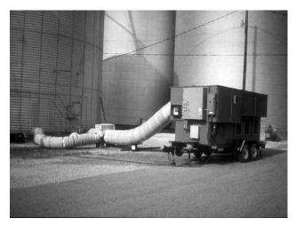
Figure 1. Grain chillers rom Burks et al. 2000).
