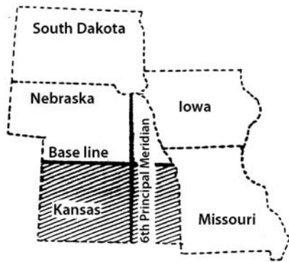
Map showing areas governed by the sixth principal meridian and its base line.
