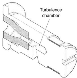
*Pre-orifice flood nozzle with turbulence chamber*
