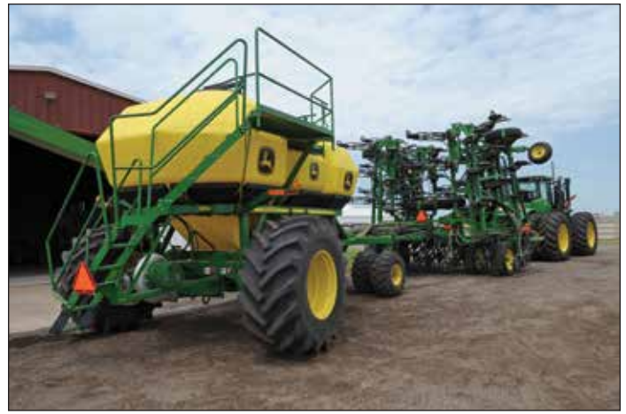
Schrock's John Deere 1870 hoe drill is used for canola, double-cropped grain sorghum, wheat, and sesame.
