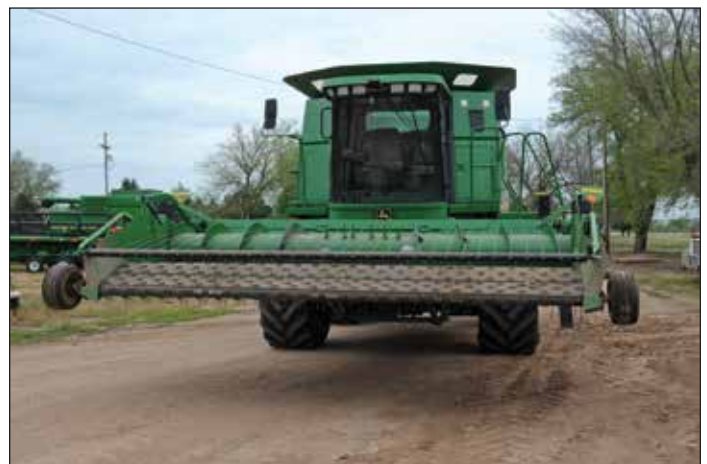
Turek invested in some equipment such as this pick up header to harvest his canola.
