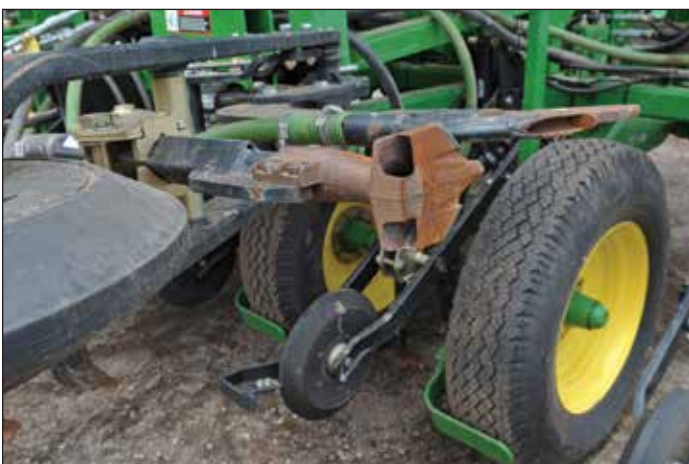
The paired row setup for the John Deere 1870 is pictured here. The fertilizer shank runs in front of the seed tube.
