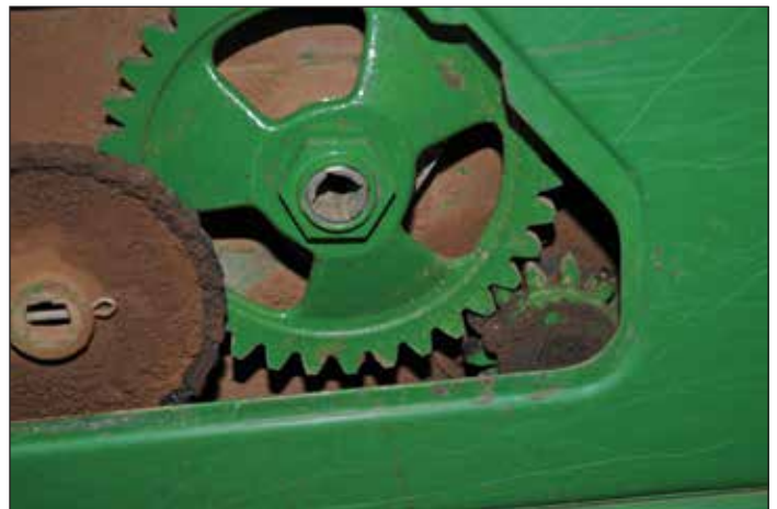
A half-speed kit was needed on the drill to slow it down enough for canola seed.
