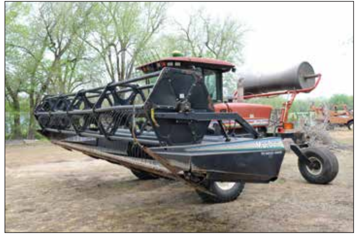
Turek uses a draper swather with a roller attachment to prepare his canola for harvest.
