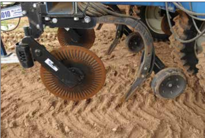
Schrock uses a Blue-Jet no-till anhydrous ammonia applicator with a coulter, mini mole knife, and press wheel on 20-inch centers.
