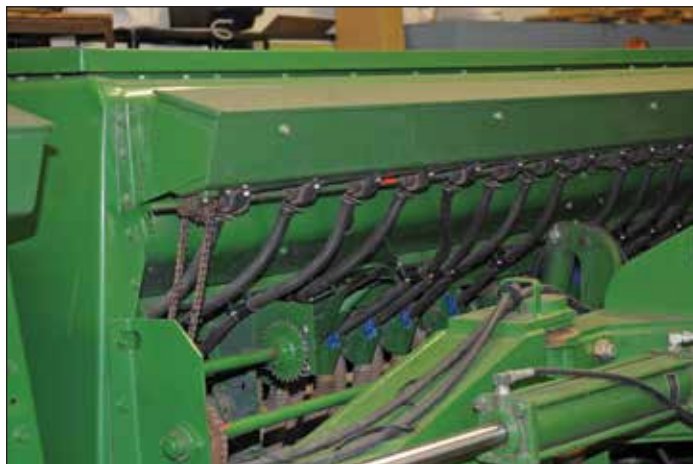
Swinehart uses a John Deere 455 drill with a straight flute and grass seed boxes to plant canola.
