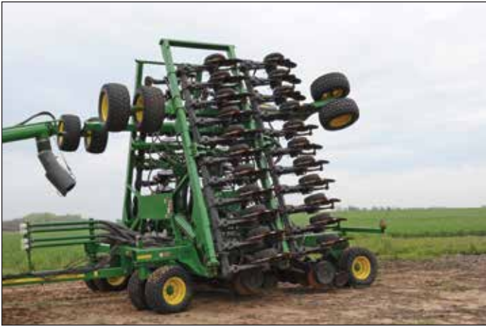
Turek's John Deere 1890 single disk no-till air drill does a good job of seed placement.
