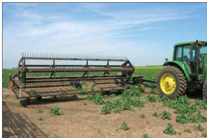
Schrock has used pull type draper swathers with roller attachments to prepare his canola for harvest.
