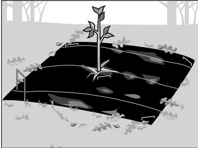
Figure 5. Five staples are used to hold fabric squares down.
