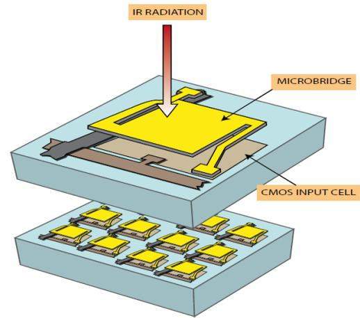
Figure 3. Schematic overview of a microbolometer detector (source: FLIR Technical Note).
