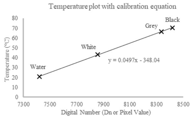
Figure 4. Thermal infrared imagery calibration setup and a sample calibration curve.
