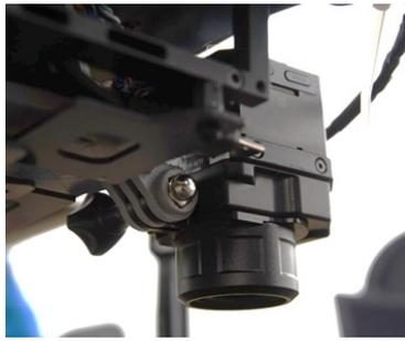
Figure 2. Uncooled thermal infrared sensor mounted on an UAV.
