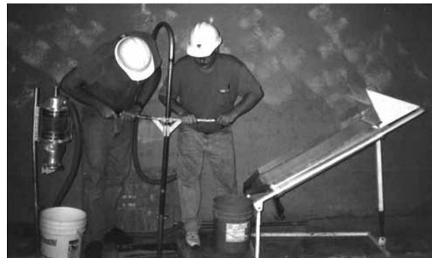
**Figure 2.** A vacuum probe system can be used to sample grain in elevator bins and an inclined sieve can be used to separate insects from large grain samples.
