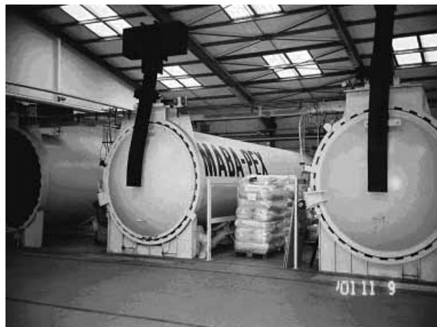
**Figure 2.** Application of high pressure CO<sub>2</sub> for the dry fruit industry in Turkey.
