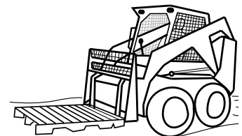
CARRYING THE ATTACHMENT AS LOW TO THE GROUND AS POSSIBLE.
