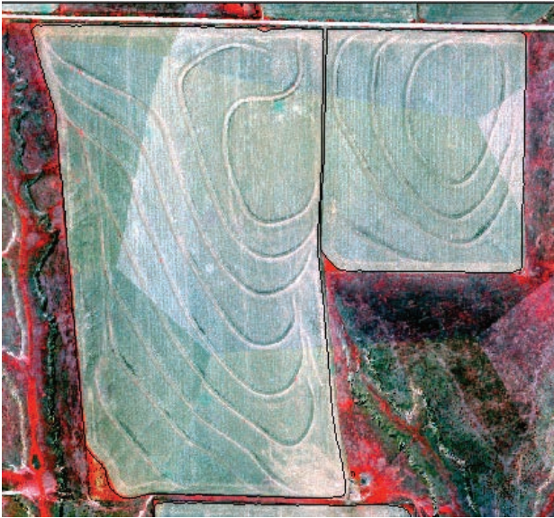
Figure 1. April 13, 2000, image for fields in northwest Kansas*. This false color composite was created using spectral bands 4 (NIR), 3 (red), 2 (green) and assigned to the red, green and blue color areas of the computer monitor.
