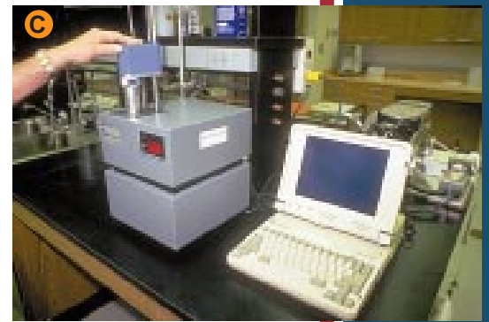
A Single kernel wheat characterization system
