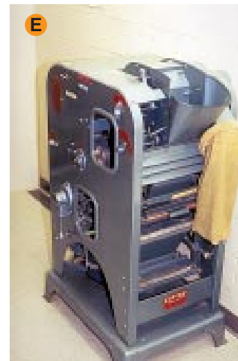
A Single kernel wheat characterization system
