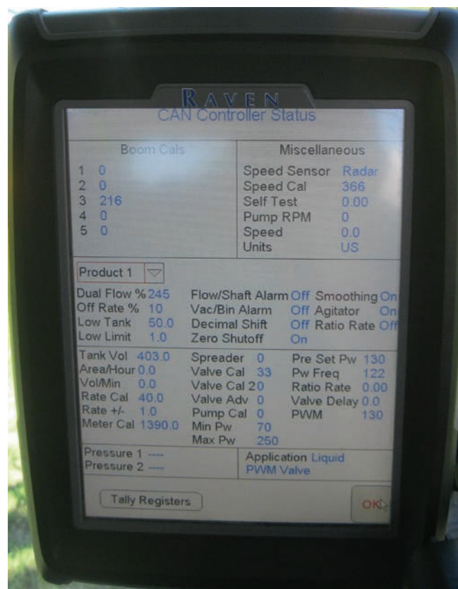
Figure 8. PWM product flow control valve setting page in the Raven Viper Pro rate controller.
