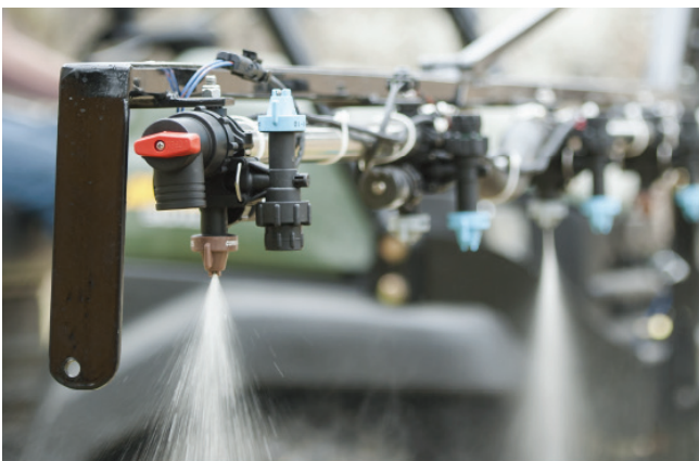
Figure 5. Odd nozzle spraying and even nozzles off during application.
