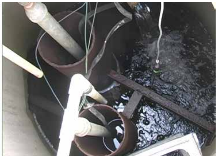
Figure 4.6. The gas monitor at left shows just 16.6% oxygen in the air of the irrigation water structure at right. Normal air contains 20% to 21% oxygen. Concentrations below 19.5% are oxygen deficient and potentially hazardous.
