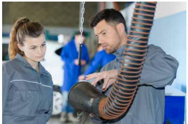
Figure 7.9. Tailpipe-exhaust extraction systems can be clamped to the tailpipe of machinery during maintenance and repair in indoor spaces.
