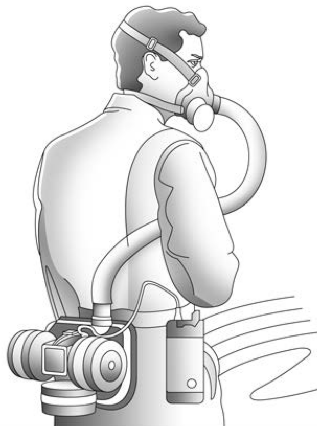
Figure 12.5. Half-face PAPR. (Credit: OSHA)
