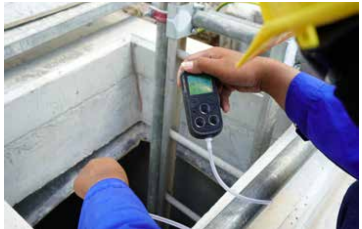
Figure 11.9. Monitor the air before and during entry to permit-required confined spaces.
