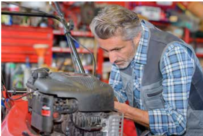
Figure 7.4. Small engines can create hazardous levels of carbon monoxide while running in repair shops and other indoor spaces.
