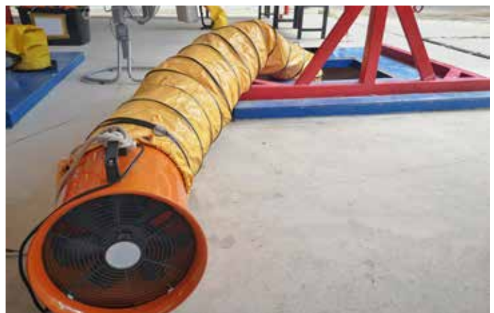
Figure 11.10. Ventilate, if necessary, to reduce airborne hazards.
