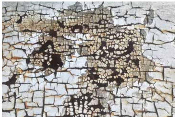
Figure 10.2. Lead-based paint can release harmful dust when scraped or sanded. (Credit: Agricultural Research Service)
