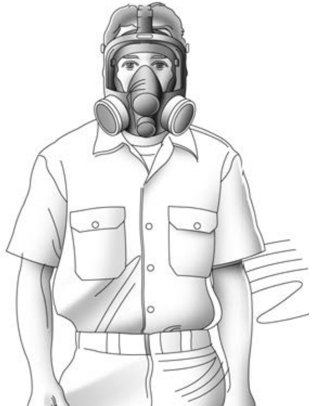
Figure 12.3. Full-face air-purifying respirator. (Credit: OSHA)
