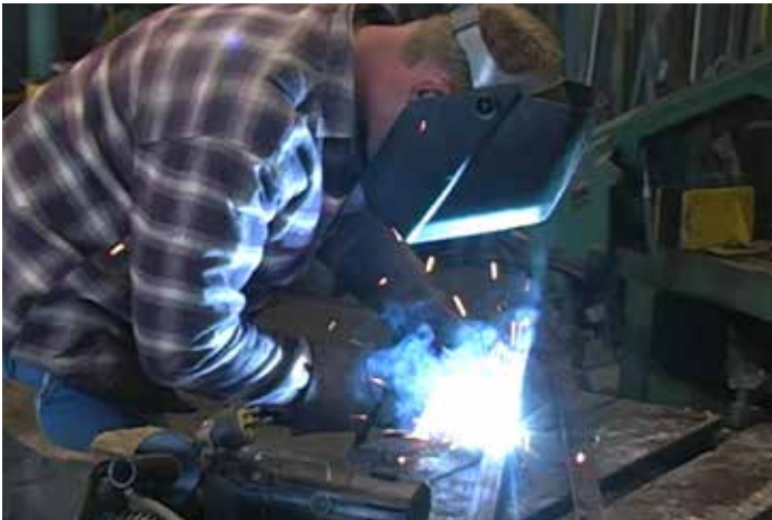
Figure 8.1. Welding, torch-cutting, and other hot work expose farmers to various fumes and gases. Some can be harmful, especially in poorly ventilated areas.
