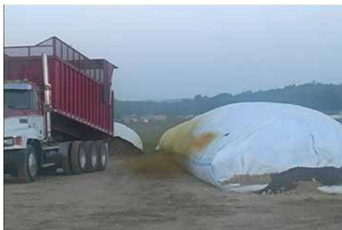
Figure 4.13. Do not park near freshly filled silage structures. Drifting toxic gases may prevent access to the vehicle.
