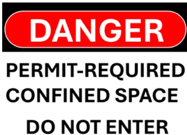
Figure 11.8. Use signs and barriers to keep unauthorized people out of permit-required confined spaces.
