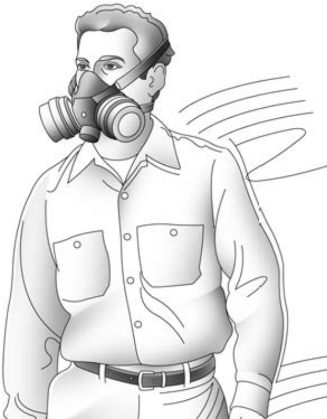
Figure 12.2. Half-face air-purifying respirator. (Credit: OSHA)
