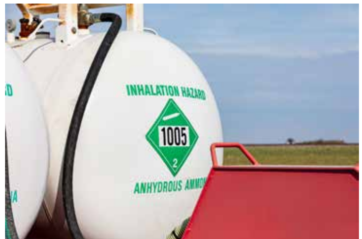
Figure 6.3. Wear protective equipment and follow the tank manufacturer's instructions when attaching or removing anhydrous ammonia hoses.
