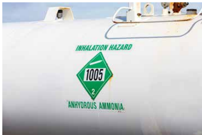
Figure 6.2. Pressurized anhydrous ammonia can cause severe chemical burns to the respiratory system, eyes, mouth, and skin.
