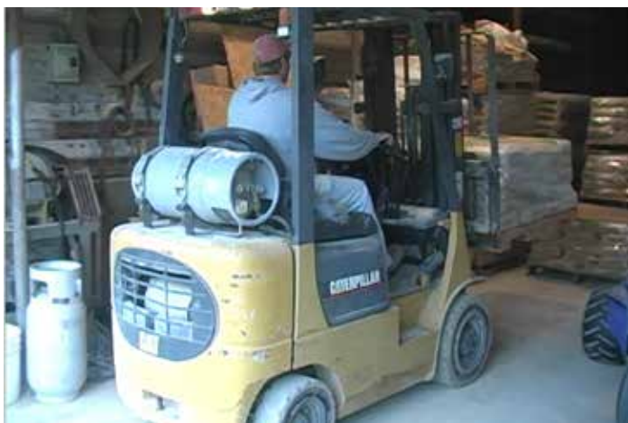
Figure 7.1. Combustion engines, such as the propane engine of this forklift, emit carbon monoxide, oxides of nitrogen, and other hazardous gases in poorly ventilated buildings and trailers.
