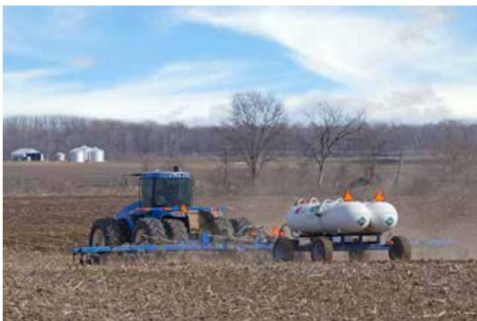
Figure 6.1. Hoses deliver anhydrous ammonia fertilizer from the white field tanks to the blue application toolbar behind this tractor.
