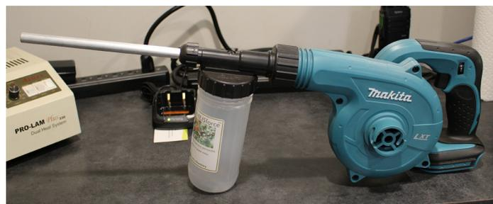
**Figure 4.** Mechanical blower used to distribute *Neoseiulus cucumeris* in a greenhouse (Photo: Raymond Cloyd).
