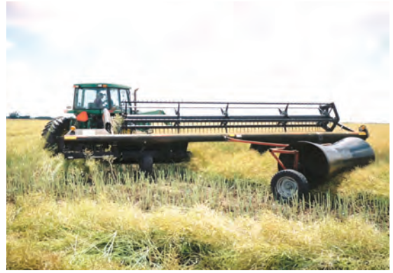
Photo 102. Swathing with roller attachment.
