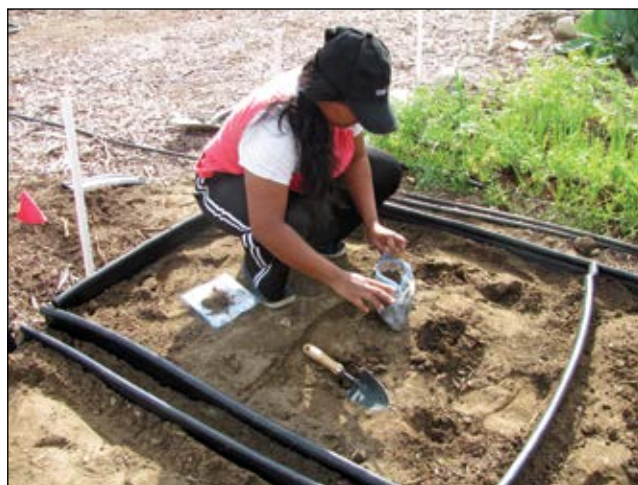
Soil should be sampled to a 6-inch depth and placed in a resealable plastic bag.
