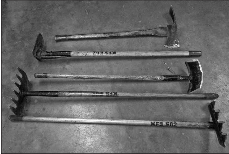
Pulaskis, combi tools, Rhinos, McCleods, and council rakes (top to bottom) are all useful tools for establishing control lines in timber fires
