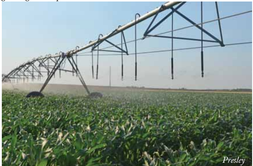
Figure 18. A modern center pivot irrigation system delivers water to a growing corn crop.
