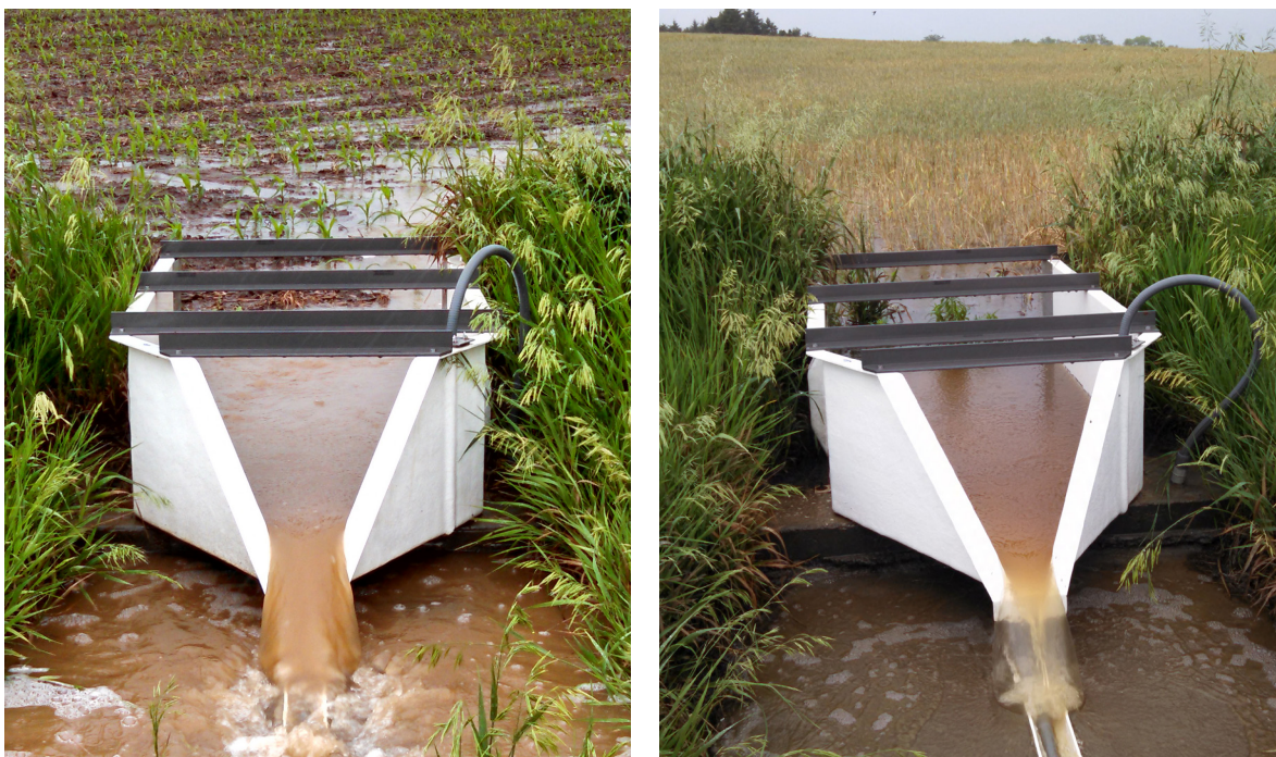
Figure 2. A May 2017 runoff event from a non-cover-crop plot (left) and a cover-crop plot (right) in a corn production year. Runoff water from the cover-crop plot is clearer than the no-cover-crop plot, visually indicating reduced sediment loss with the cover crop.
