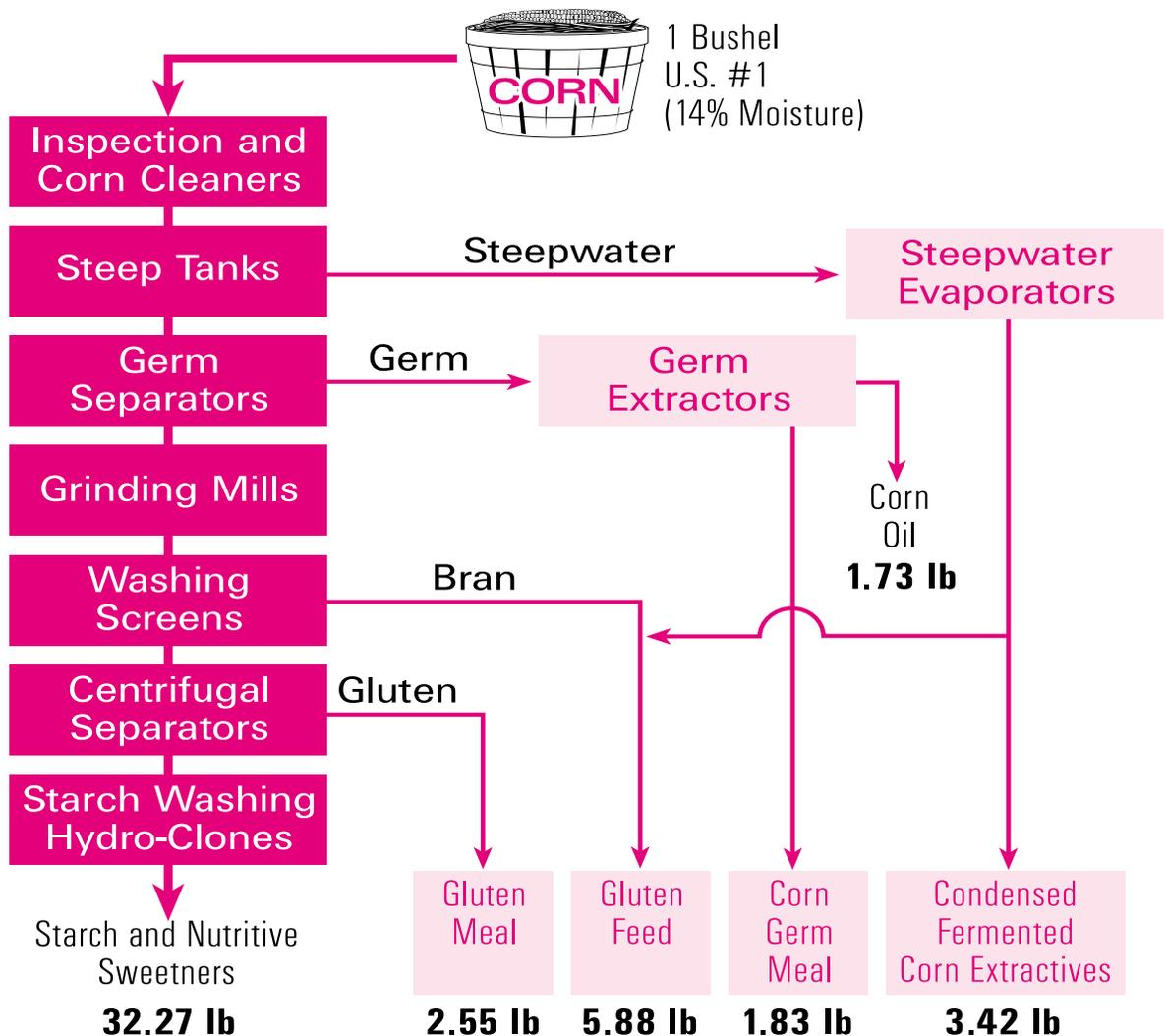
**Stage 3. Fine Grinding and Screening**—The corn and water slurry exits the germ separator for a more concise grinding in an impact or attrition-impact mill to release the starch and gluten from the fiber in the kernel. The fiber fraction is collected, slurried, and rescreened again to reclaim residual starch or protein and passed on to the mill stream destined for animal feeds. The separated starch/gluten suspension (often referred to as mill starch) is transported to the starch separators.
