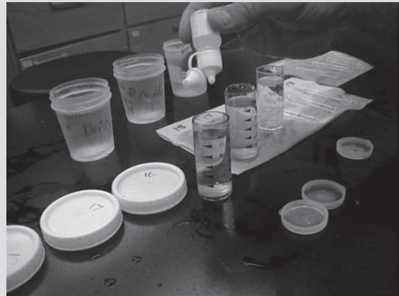
Figure 5-2. Add 25 ml of water to sample vial, then add two drops of activator solution.
