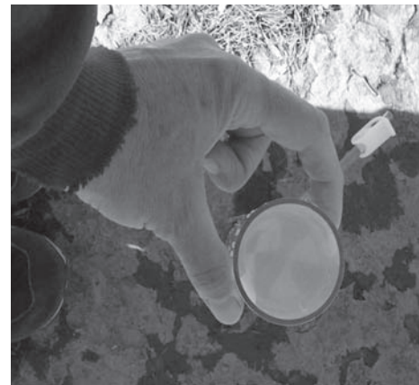
Figure 3-2. When the Secchi disk icon becomes visible, stop the flow of water and take the reading from the side of the tube in centimeters.
