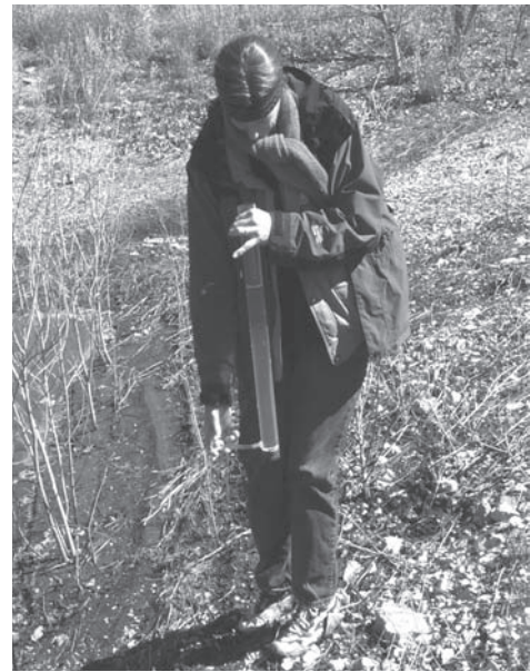
Figure 3-1. Read the transparency tube while looking at the Secchi disk icon at the bottom.
