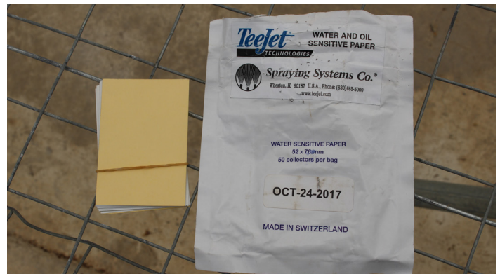
Figure 9. Water sensitive spray cards can be used to assess the coverage of plants with insecticide spray applications (Photo: Raymond Cloyd).
