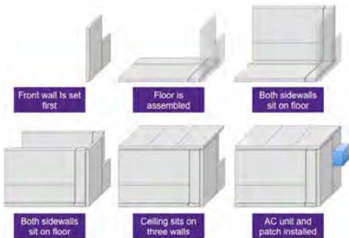
Figure 3. A diagram showing the arrangement and order for installing structurally insulated panels (SIPs) in the mobile cooler.
