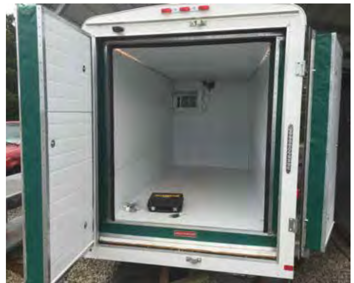
Figure 13. The cooler complete with trim and weather-stripping.
