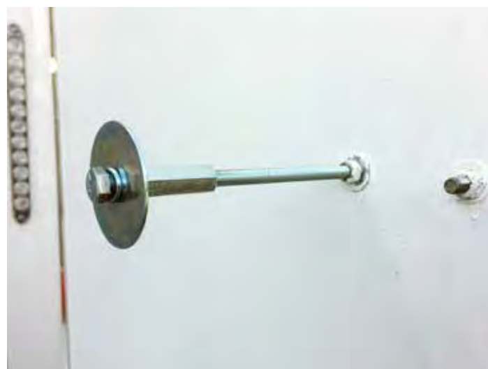
Figure 11. Hardware used to mount the 6-inch insulated panel to the trailer doors. Replace one bolt at each hinge and one at the latch for each door.
