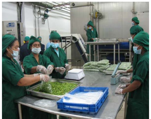
Blanched long bean (Lubea) being packaged and weighed prior to deep freezing at the Golden Harvest agro processing plant in Gazipur, Bangladesh.
