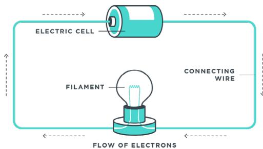
The electrical current's path of circuit is considered to be closed if electrons are allowed to flow completely through the cycle. An electric circuit is considered open if the electrical path is broken and electrons are not allowed to flow to complete the cycle.
